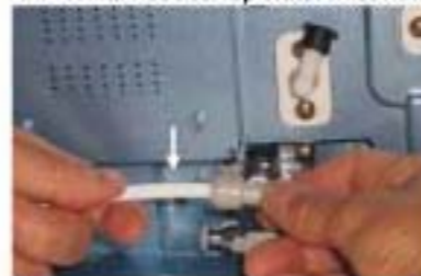
1/4" White hose to Tap Water Inlet Port
