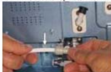
1/4" White hose to Tap Water Inlet Port
