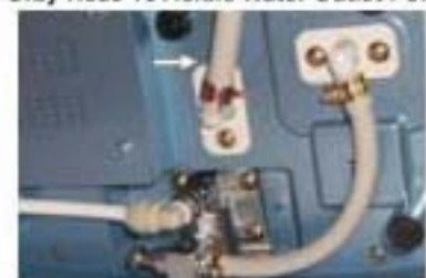
Gray Hose To Acidic Water Outlet Port
