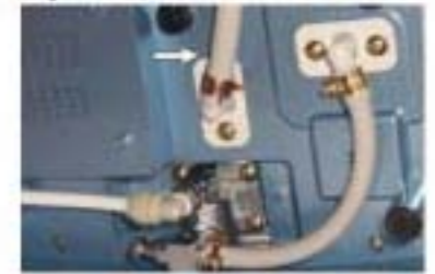
Gray Hose To Acidic Water Outlet Port
